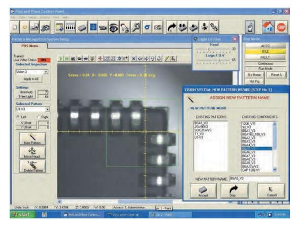
The vision software is Windows® based to allow easy straightforward teach-in, requiring minimal operator training.
