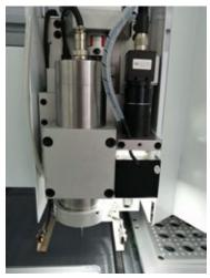
400W high-power spindle, which can cut Al board below 2.0mm thickness (machine needs to use custom-cut aluminum board milling cutter)
