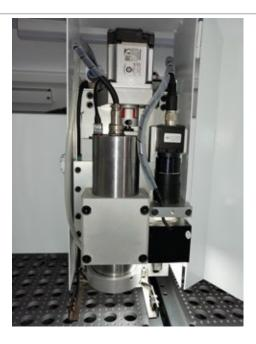
Equipped with High resolution CCD makes programming very easy. It has mark positioning function ,can automatically correct the coordinate offset. Also the CCD has the function of scanning bar code and QR code, which can scan the bar code and QR code information on the PCB board directly, and then call the finished program on the machine to cut the PCB board directly.
